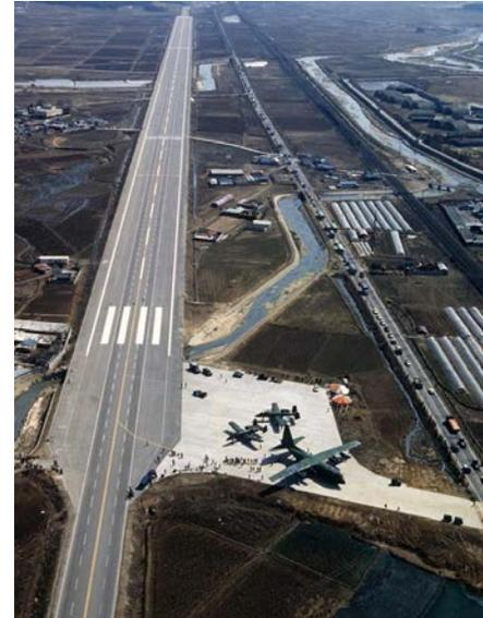
Figure 1: Expressway 1 in South Korea, which has a built-in airfield. Military planes are practicing landing and taking off from it during an exercise.<sup>[7]</sup>
